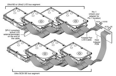
Figure 3. Cable connections and external termination
